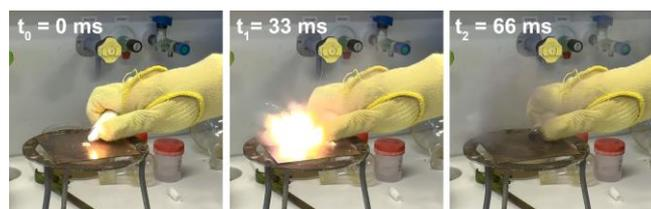
**Figure 14.** Initiation of silver 1-oxido-5*H*-tetrazolate (**4**) by a lighter.  $t_0$ ) right before the flame is in contact with the compound;  $t_1$ ) immediate detonation of **4** on contact with the flame;  $t_2$ ) smoke residue after detonation.
