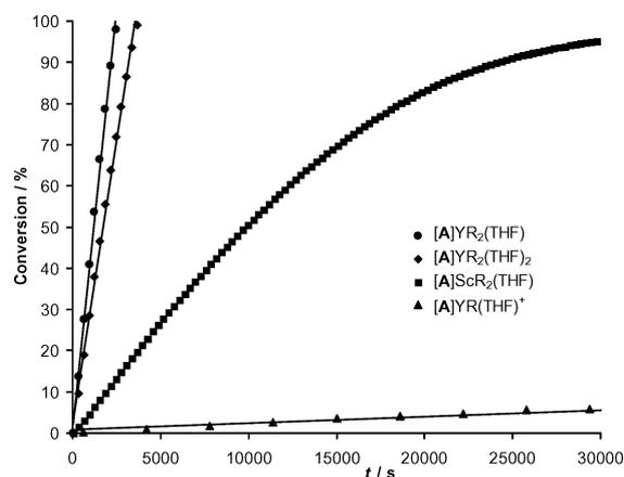
**Fig. 1** Hydroamination/cyclisation of 2,2-dimethyl-4-pentenylamine with  $[\text{A}]\text{YR}_2(\text{THF})_n$  ( $n = 1, 2$ ),  $[\text{A}]\text{ScR}_2(\text{THF})$  and  $\{[\text{A}]\text{YR}(\text{THF})\}^+$  catalysts in  $\text{C}_6\text{D}_6$ . A conversion of 100% corresponds to 100 turnovers.
