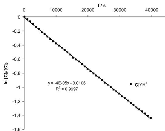
**Fig. 3** Plot showing first order substrate concentration dependence of the hydroamination/cyclisation of 2,2-dimethyl-4-pentenylamine by  $\{[C]YR\}^+$  catalyst in  $C_6D_6$  solvent at 50 °C.
