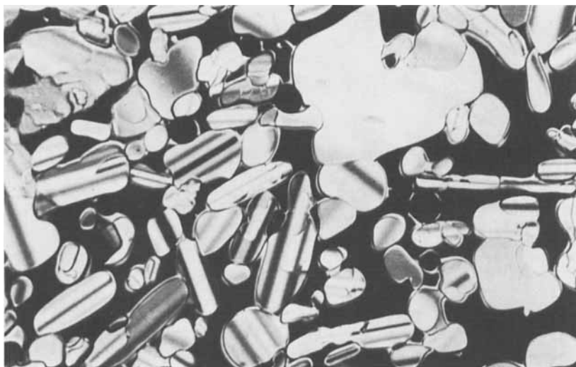
FIGURE 3 S_B - N transition for 4-propionyl-4'-ethanoyloxyazobenzene ( n = 0 ) observed at 402°K during heating of the sample. Film between glass slides, crossed polarizers, magnification 80x.
