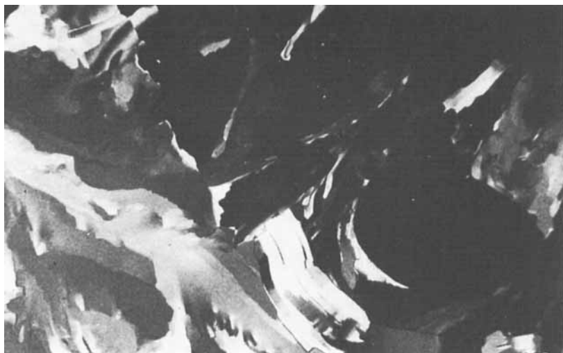
FIGURE 7c Photomicrographs of 4-propionyl-4'- n -pentanoyloxyazobenzene ( n = 3 ), crossed polarizers, magnification 80\times , cooling cycle. Texture of S_B phase at 365.5^\circ\text{K} .
