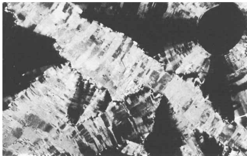
FIGURE 8b Photomicrographs of 4-propionyl-4'- n -hexanoyloxyazobenzene ( n = 4 ) taken during a cooling cycle, crossed polarizers, magnification 80\times . Broken focal conic fan texture of S_C phase.
