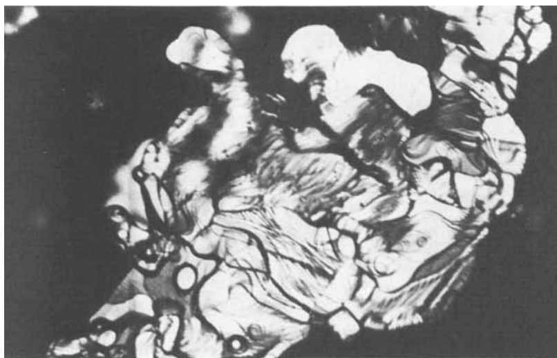
FIGURE 4 Smectic B phase of 4-propionyl-4'-propanoyloxyazobenzene ( n = 1 ). Photomicrograph taken at 405°K during an heating cycle performed on a sample previously kept at 404°K for one hour. Film between glass slides, crossed polarizers, magnification 120x.
