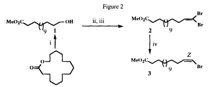
Reaction conditions : (i) MeOH, APTS cat. 12h, reflux; (ii) PDC,  $CH_2Cl_2$ , (iii) PPh<sub>3</sub>,  $CBr_4$ , Zn, THF, 80 % for the three steps; (iv) *n*-Bu<sub>3</sub>SnH, Pd(PPh<sub>3</sub>)<sub>4</sub>, 83 %
