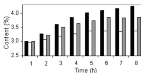
Fig. 2. Water content of the reaction mixtures without water removal (black columns), using pervaporation (white columns), and using zeolite adsorption (gray columns) (solvent: Cyphos 202;  $T = 40^\circ\text{C}$ ).
