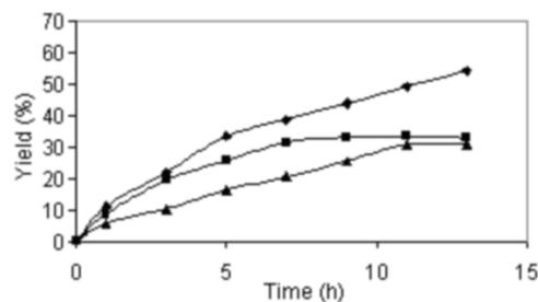
Fig. 1. Effect of water removal on ethyl lactate yield without water removal (◆), with pervaporation water removal (■), and with water removal by adsorption (zeolite) (▲) (solvent: Cyphos 202;  $T = 40^\circ\text{C}$ ).
