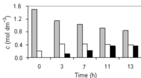
**Fig. 3.** Concentrations of lactic acids and ethyl lactate in the reaction mixture using water adsorption by zeolite: LA content (gray columns), LA<sub>2</sub> content (white columns), and ester content (black columns); solvent: Cyphos 202;  $T = 40\text{ }^{\circ}\text{C}$ .
