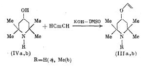
The following conditions turned out to be the best: a KOH-DMSO system, temperature 90°C, KOH concentration 20% based on the weight of (VIa), time 3-4 h. Acetylene was passed into an autoclave at an initial pressure of 10-14 atm until the solution was saturated. The yield of ether (IIIa) was 70%. According to the physical constants, IR and PMR spectra, the vinyl ether obtained was identical to the reduction product formed when nitroxyl (I) was vinylated.
