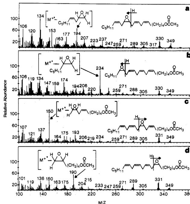
Figure 2. Carbon disulfide charge exchange mass spectra of the monoepoxide isomers of arachidonyl acetate.
