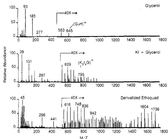
**Figure 4.** Comparison of the positive ion spectra of glycerol (top), KI plus glycerol (center), and Ethoquad 18/25 derivatized with perfluorooctanoic anhydride (bottom) under identical instrument conditions.
