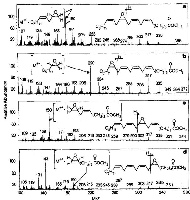
**Figure 3.** Carbon disulfide charge exchange mass spectra of the monoepoxide isomers of methyl arachidonate.
