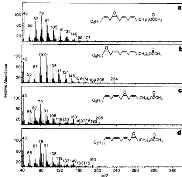
Figure 1. Electron ionization (70 eV) mass spectra of the monoepoxide isomers of arachidonyl acetate.
