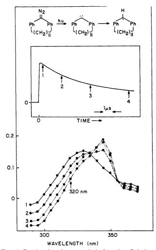
Figure 1. Transient absorption spectra obtained upon laser flash photolysis of diazo compound 4b in argon-purged hexane. Also shown is the time-resolved behavior observed at 320 nm. The four spectra were recorded at the four times after the laser pulse indicated on the decay trace.
