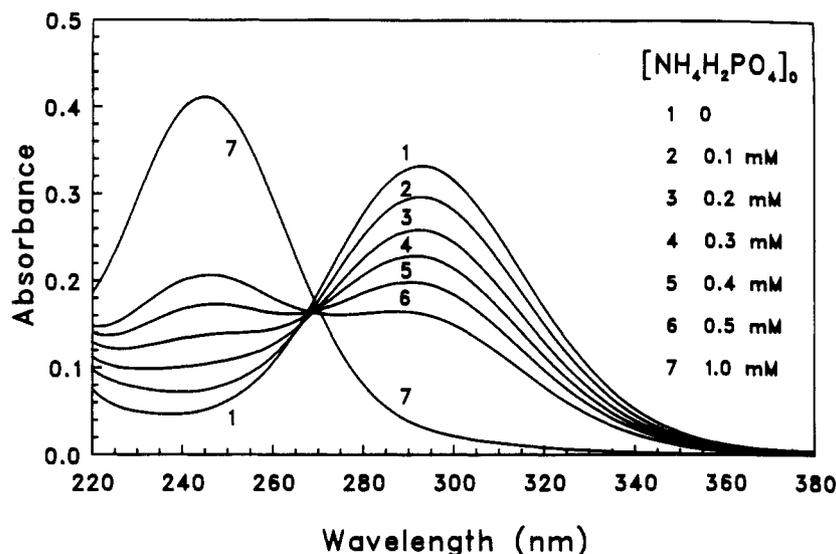
**Figure 9.** UV spectra of solutions containing various initial concentrations of  $\text{NH}_4\text{H}_2\text{PO}_4$  (0–1 mM) and 1 mM HOCl in 40 mM  $\text{Na}_2\text{B}_4\text{O}_7$  (pH 9.1). Spectra demonstrate the presence of only  $\text{OCl}^-$  ( $\lambda_{\text{max}}$  292–294 nm) and  $\text{NH}_2\text{Cl}$  ( $\lambda_{\text{max}}$  244 nm).
