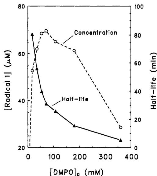
**Figure 11.** The initial concentration and half-life of 1 in solutions containing 2 mM  $\text{NH}_4\text{H}_2\text{PO}_4$ , 4 mM  $\text{HOCl}$ , 18–359 mM  $\text{DMPO}$ , and 40 mM  $\text{Na}_2\text{B}_4\text{O}_7$  (pH 9.1). The concentrations of 1 were obtained by extrapolating the decay curves to zero time.
