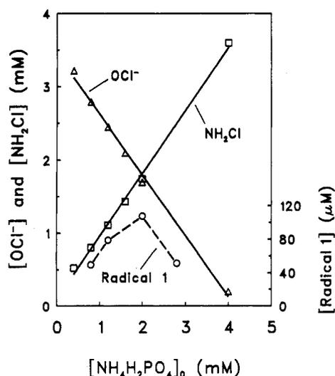
**Figure 10.** Correlation of the maximum concentration of initial 1 (from Figure 8) with the concentrations of  $\text{NH}_2\text{Cl}$  and  $\text{OCl}^-$  corresponding to various initial concentrations of  $\text{NH}_4\text{H}_2\text{PO}_4$  at pH 9.1.<sup>36</sup> For further details, see legend to Figure 8.
