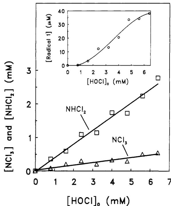
**Figure 2.** Concentrations of  $\text{NCl}_3$  and  $\text{NHCl}_2$  in solutions that contained various initial concentrations of HOCl (0.8–6.4 mM) and 40 mM  $\text{NH}_4\text{H}_2\text{PO}_4$  in 40 mM  $\text{KH}_2\text{PO}_4$ – $\text{H}_3\text{PO}_4$  (pH 3). Inset: Concentration of the radical 1 estimated from EPR spectra recorded 0.6 min after the addition of DMPO (72 mM) to the above solutions.
