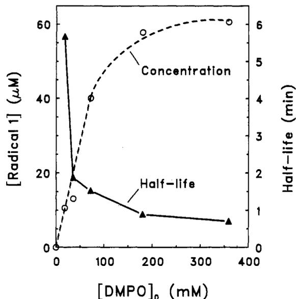
**Figure 5.** The initial concentration and half-life of 1 corresponding to various concentrations of DMPO (18–359 mM), 40 mM  $\text{NH}_4\text{H}_2\text{PO}_4$ , 4 mM HOCl, and 40 mM  $\text{KH}_2\text{PO}_4\text{--H}_3\text{PO}_4$  (pH 2.8). The concentrations of 1 were obtained by extrapolating the decay curves to zero time.
