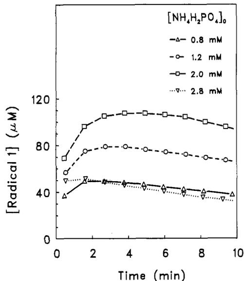
**Figure 8.** Time course of 1 formed in solutions containing various initial concentrations of  $\text{NH}_4\text{H}_2\text{PO}_4$  (0.8–2.8 mM), 4 mM HOCl, 72 mM DMPO, and 40 mM  $\text{Na}_2\text{B}_4\text{O}_7$  (pH 9.1).
