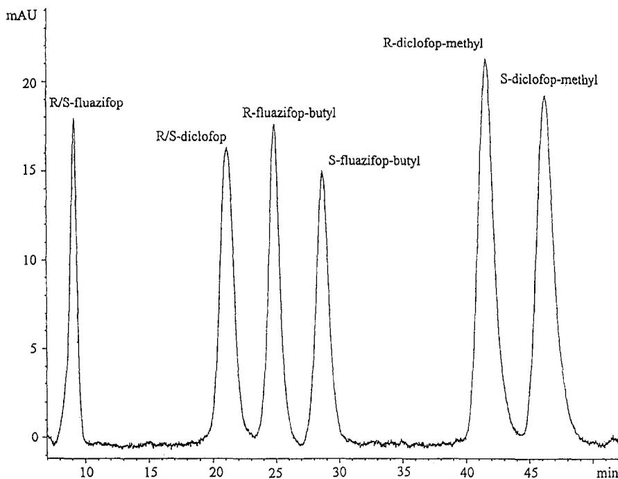
**Figure 1:** Separation of fluazifop, diclofop and the enantiomers of corresponding esters using chiral permethylated  $\beta$ -cyclodextrin HPLC column (eluent: 70 % methanol buffered at pH 4 with 0.4 % triethyl ammonium acetate, flow rate: 0.4 mL/min, injection volume: 20  $\mu$ L, detection: 233 nm).
