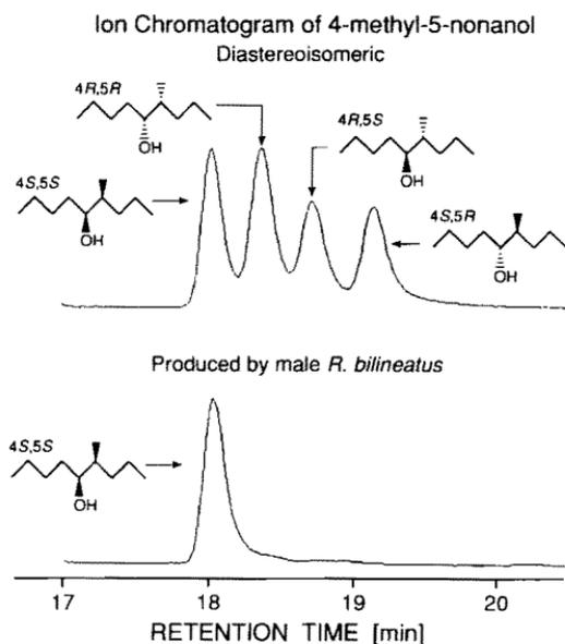
FIG. 3. Selected ion  $m/z = 69, 87,$  and  $101$  chromatogram (Hewlett Packard 5985B GC-MS) of stereoisomeric and weevil-produced **1**.  $m/z$  was the parent ion of the full scan EI mass spectrum of  $(M^+ - C_4H_9)$   $101$  or  $(M^+ - C_5H_{11})$   $87$ . Analysis on a Cyclodex B column, isothermal  $100^\circ\text{C}$ , linear flow velocity of carrier gas  $35\text{ cm/sec}$ , split injection and injector temperature  $220^\circ\text{C}$ .
