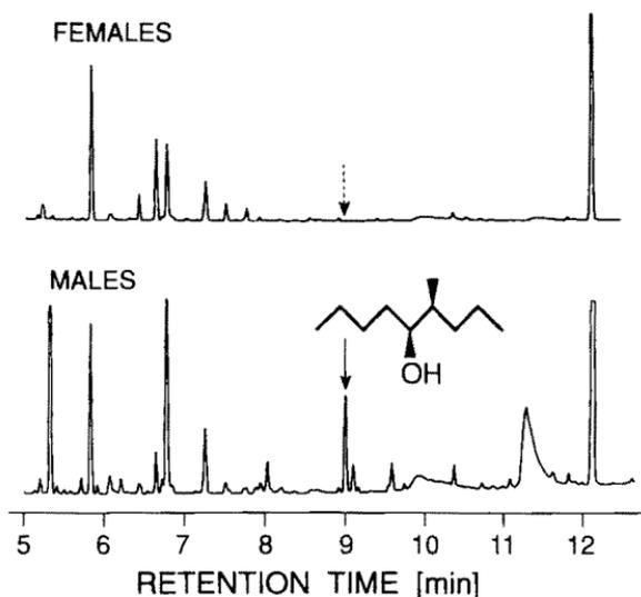
FIG. 1. Gas chromatograms of volatiles obtained from female and male *R. bilineatus* feeding on apples. Chromatography: SP-1000 fused silica column; temperature program: 1 min at 50°C, 10°C/min to 180°C.
