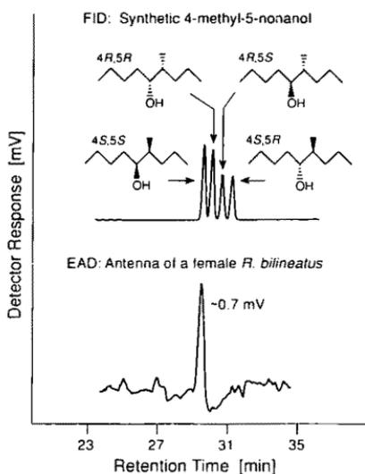
FIG. 4. Flame-ionization (FID) and electroantennographic detector (EAD: female *R. bilineatus* antenna) responses to isomers of 4-methyl-5-nonanol. Column as in Figure 3.
