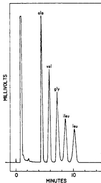
Figure 1. Separation of five *n*-butyl *N*-acetyl amino acid esters (Barber-Colman Model 10)
