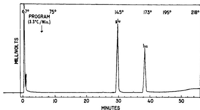
Figure 4. Chromatogram of the *n*-butyl *N*-trifluoroacetyl ester prepared from lysine with glutamic acid as an internal standard (F and M Model 400)
