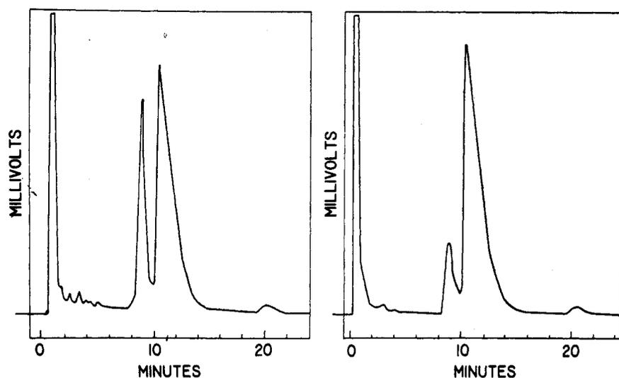
Figure 2. Thermal decomposition of the *n*-butyl *N*-trifluoroacetyl ester of threonine as influenced by flash-heater temperature (F & M Model 1609)
