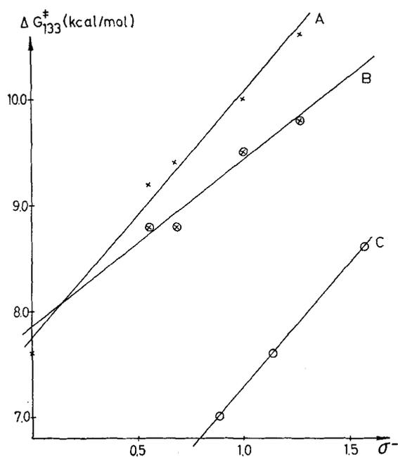
FIG. 2. Hammett correlations. Barriers ( $\Delta G_{133}^\ddagger$ ) vs.  $\sigma^-$  values.
