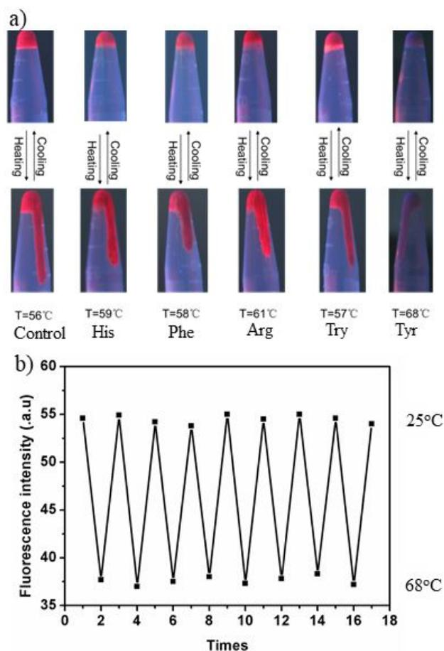
**Figure 4.** a) The amino acid-doped CdSe-LQDs exhibited excellent fluidity after heating and only the fluorescence intensity of Tyr-doped nanofluids was almost completely quenched. b) The cycling experiment of Tyr-doped CdSe-LQDs from heating and cooling.
