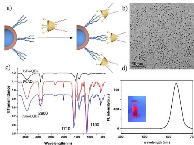
**Figure 2.** a) A schematic illustration of preparing CdSe-LQDs via hydrophobic interaction. b) TEM image of CdSe-LQDs. c) IR spectrum of CdSe-QDs, PCAD and CdSe-LQDs. d) Fluorescence emission of CdSe-LQDs.
