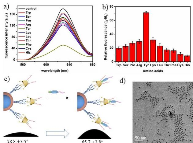
**Figure 3.** a) Fluorescence spectra showing the response of CdSe-LQDs to 11 amino acids in  $\text{CH}_3\text{CN}/\text{H}_2\text{O}$ . b) Relative fluorescence intensity ( $(I_0-I)/I_0$ ),  $I_0$  and  $I$  are the fluorescence intensities without and with amino acids. c) Profiles of water droplets on the CdSe-LQDs on quartz substrates and treated with Tyr and Tyr induced CA of CdSe-LQDs change from  $28.8^\circ$  to  $65.7^\circ$ . d) TEM image of CdSe-LQDs in the presence of Tyr.
