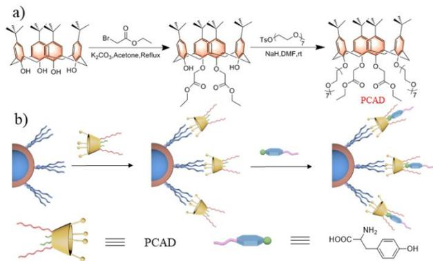
**Figure 1.** a) The synthetic scheme of PCAD. b) A schematic illustration to show that the PCAD coated on the CdSe-QDs to produce CdSe-LQDs and it responds to Tyrosine.
