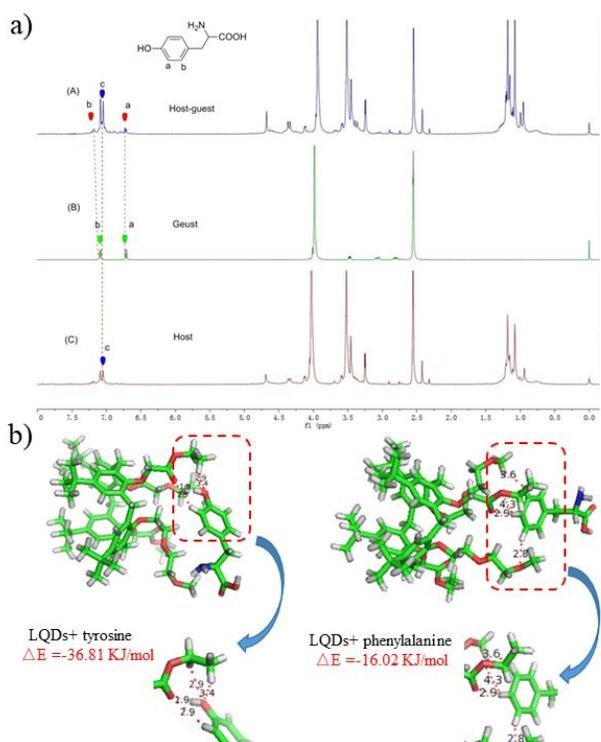
**Figure 5.** a) <sup>1</sup>H NMR spectra of (a) PCAD (5 mM) + Tyr (5 mM), (b) free Tyr (5 mM), (c) PCAD (5 mM). b) The Gaussian calculation of binding energy of PCAD + Tyr (PCAD + Phe as a control).
