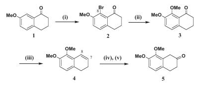
Reagents: (i) NBS, CH<sub>3</sub>CN, rt; (ii) NaOMe, CuBr, DMF-H Q, reflux; (iii) 2,4-pentanediol, *p-TsOH*, reflux; (iv) MCPBA, CH Cl 2, 0°C; (v) H<sub>2</sub>SO<sub>4</sub> (10%), EtOH
