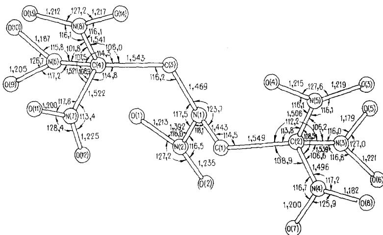
Fig. 1. Bond lengths and valence angles in the molecule of compound IA.
