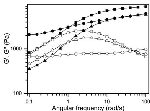
Fig. 6 Rheological oscillatory shear measurements of photo-cross-linked RGDP-PEG-acrylate<sub>6k</sub> hydrogels at various concentrations (10% w/v, squares; 8% w/v, triangles) and a covalently cross-linked control hydrogel at 8% w/v (circles). Storage modulus  $G'$ : filled symbols; loss modulus  $G''$ : open symbols. Measurements were performed at 1% strain, pH 7.4, and 37 °C.
