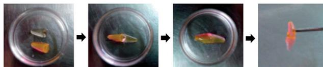
Fig. 3 Self-healing of photo-cross-linked RGDP-PEG-acrylate<sub>6k</sub> hydrogel (8% w/v) at 25 °C.
