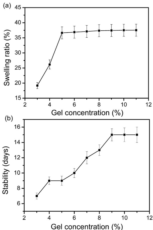
Fig. 4 Swelling ratio (a) and stability (b) of photo-cross-linked RGDP-PEG-acrylate<sub>6k</sub> hydrogels at 37 °C.
