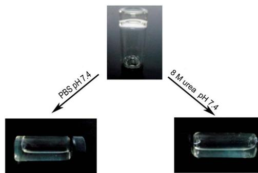
**Fig. 2** Disassembly of photo-cross-linked RGDP-PEG-acrylate<sub>6k</sub> hydrogels (8% w/w) in 0.01M PBS (pH = 7.4) and 8 M urea (pH = 7.4) at 37 °C.
