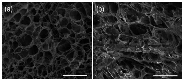
Fig. 5 SEM of photo-cross-linked RGDP-PEG-acrylate<sub>6k</sub> hydrogels: (a) 8% w/v; (b) 6% w/v. The scale bars are 40 μm.
