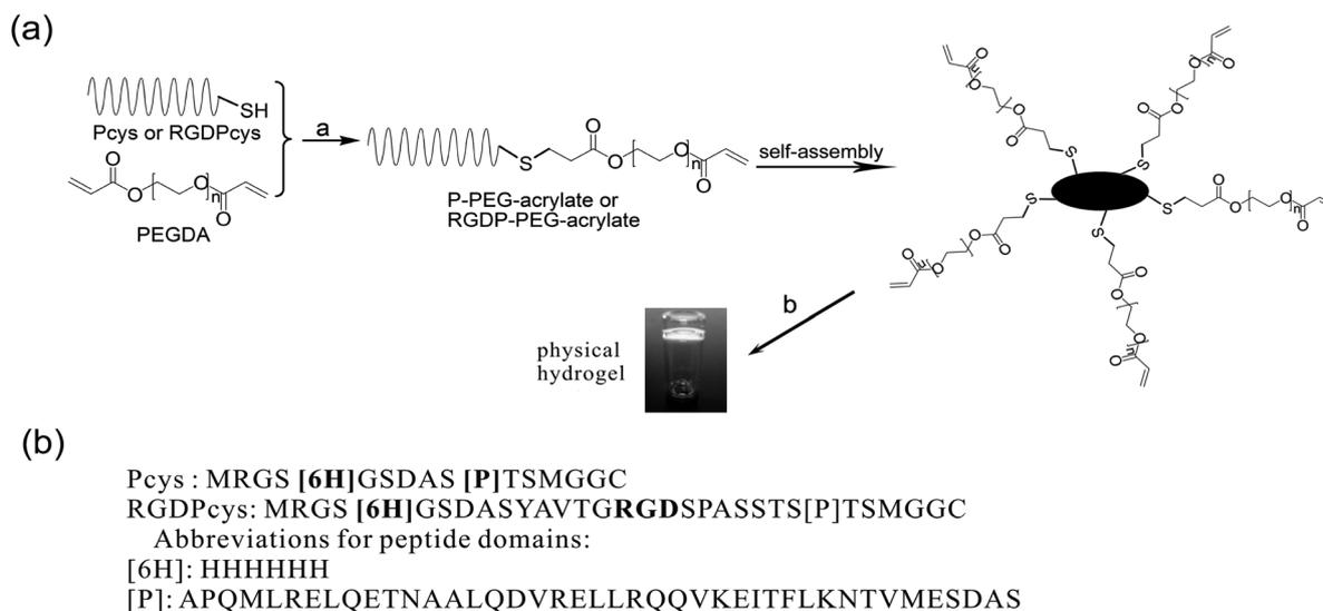
**Scheme 1** (a) Illustration of the formation of photo-cross-linkable physical hydrogels from self-assembled multi-functional macromers. (a) pH 8, 8 M urea buffer, 1.5 mM TCEP; (b) 365 nm UV light, 5 min. (b) Amino acid sequences of Pcys and RGDPcys.
