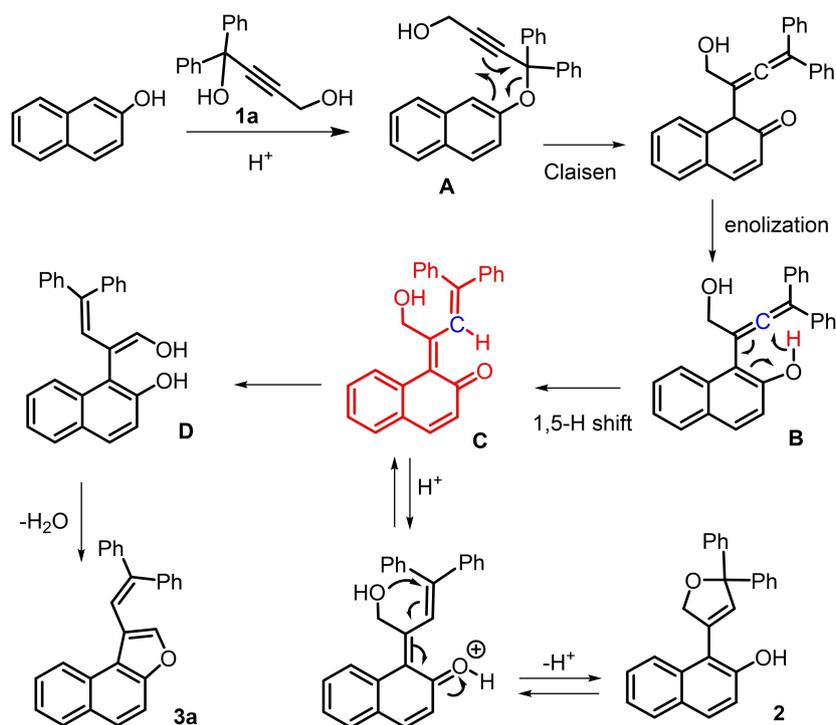
**Scheme 6.** Proposed mechanism for the reaction of 2-naphthol with 1,1-diphenylbut-2-yne-1,4-diol **1a**.
