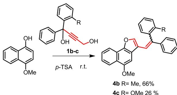
**Scheme 8.** One-pot synthesis of naphthofurans **4b–c** from 4-methoxynaphth-1-ol and 1,1-diarylbut-2-yne-1,4-diols **1b–c**.
