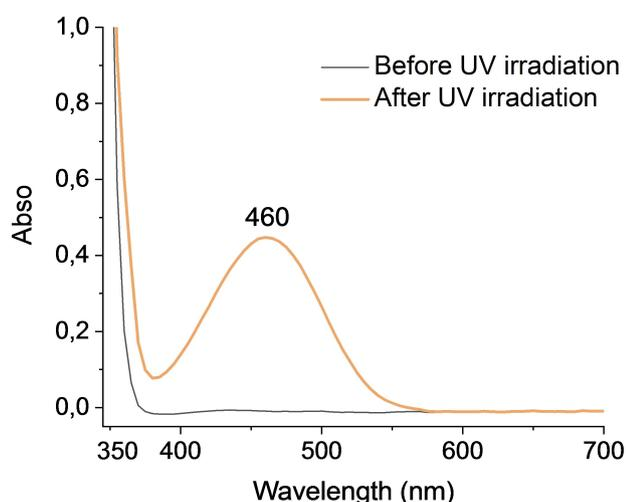
Figure 1. UV-vis spectra of vinylnaphthofuran **3a** ( $\text{CHCl}_3$ ,  $1.0 \times 10^{-3}$  M) before (black) and after exposure to the UV light (orange)
