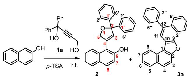
Scheme 5. Reaction of 2-naphthol with 1,1-diphenylbut-2-yne-1,4-diol **1a** at room temperature.
