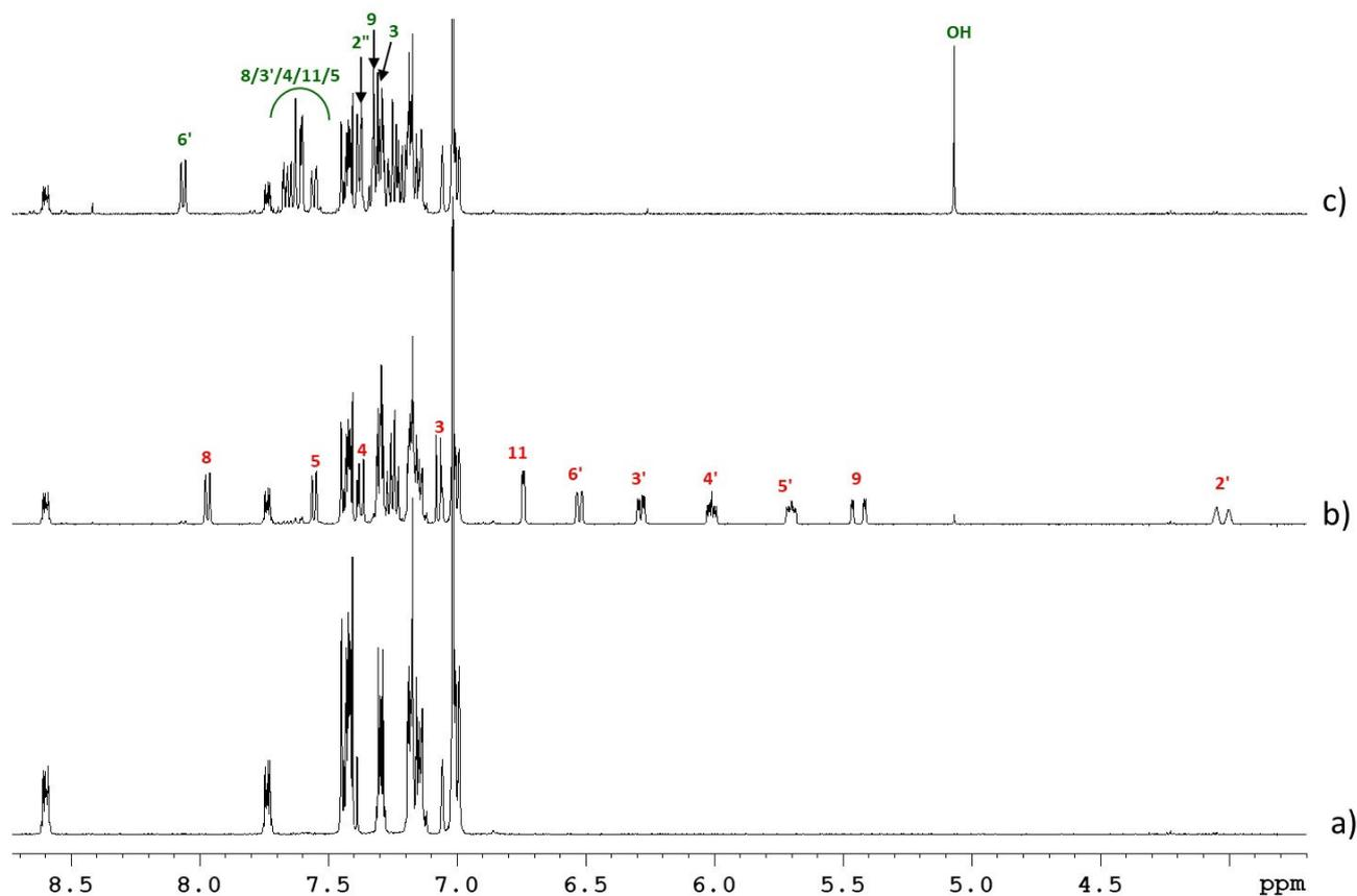
**Figure 4.**  $^1\text{H}$  NMR spectra of naphthofuran **3a** in a degassed toluene- $d_8$  solution ( $5 \times 10^{-3}$  M), a) before hv, b) after UV irradiation and c) after thermal evolution for 1 day.
