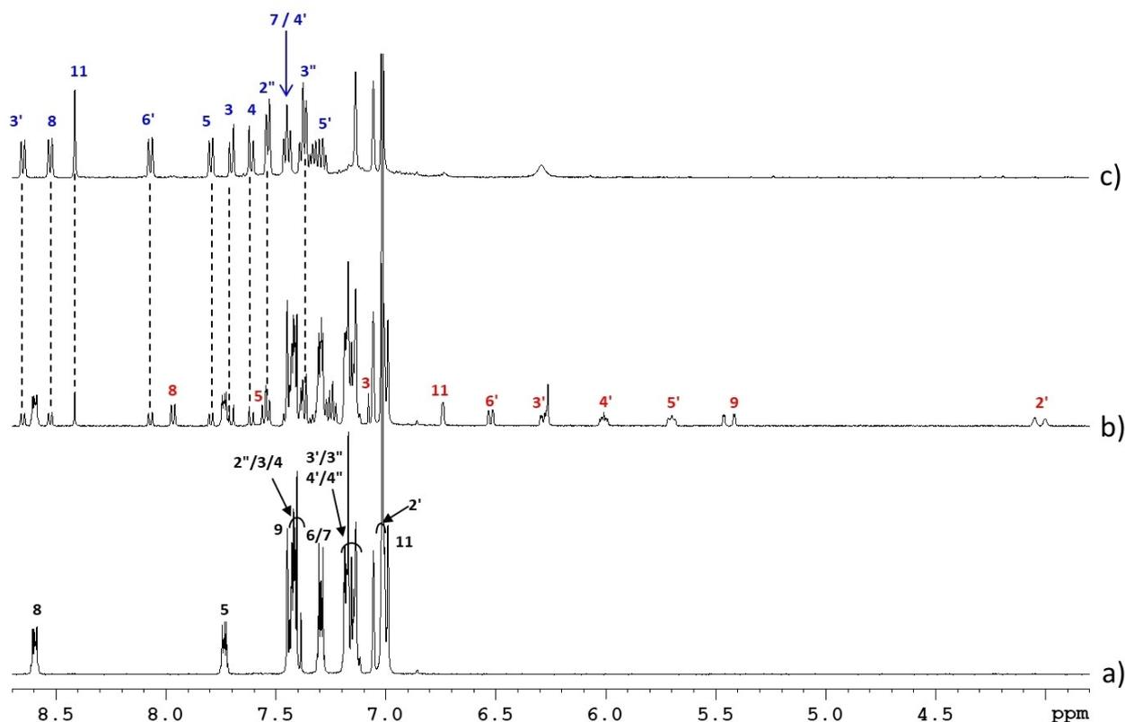
**Figure 3.**  $^1\text{H}$  NMR spectra of naphthofuran **3a** in toluene- $d_8$  ( $5 \times 10^{-3}$  M), a) before  $h\nu$ , b) after 5 min of UV irradiation at 313 nm, and c) after 20 min of UV irradiation at 313 nm. Assignment in black, red, and blue are referred to **3a**,  $\text{P}_1$  and  $\text{P}_2$ , respectively.
