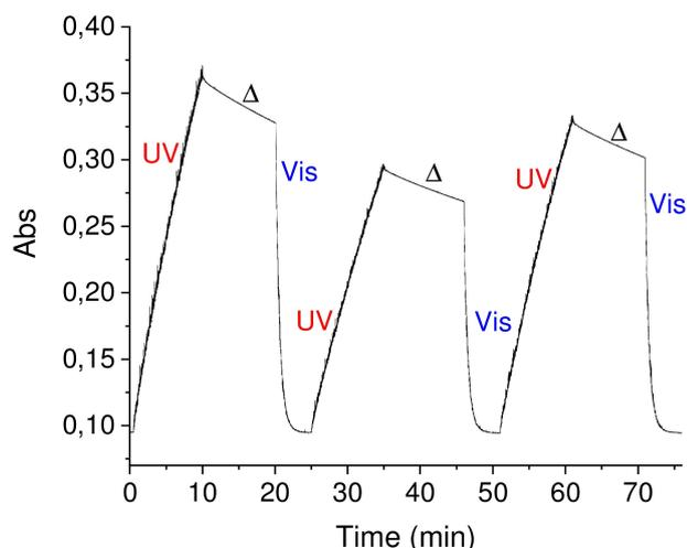
Figure 2. Successive cycles of UV/Vis irradiation for the vinylnaphthofuran **3a** in  $\text{CHCl}_3$  measured at 460 nm.
