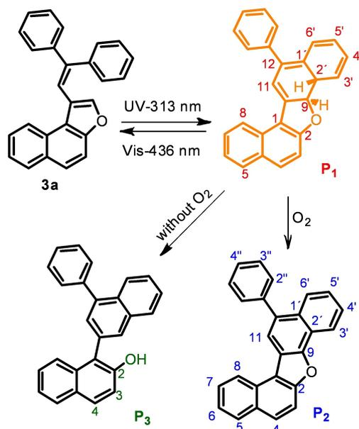
**Scheme 9.** General mechanism for the photochromic behavior of vinyl-naphthofuran **3a**.
