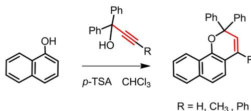
Scheme 1. Synthesis of naphthopyrans from 1-naphthol and diarylpropynols.
