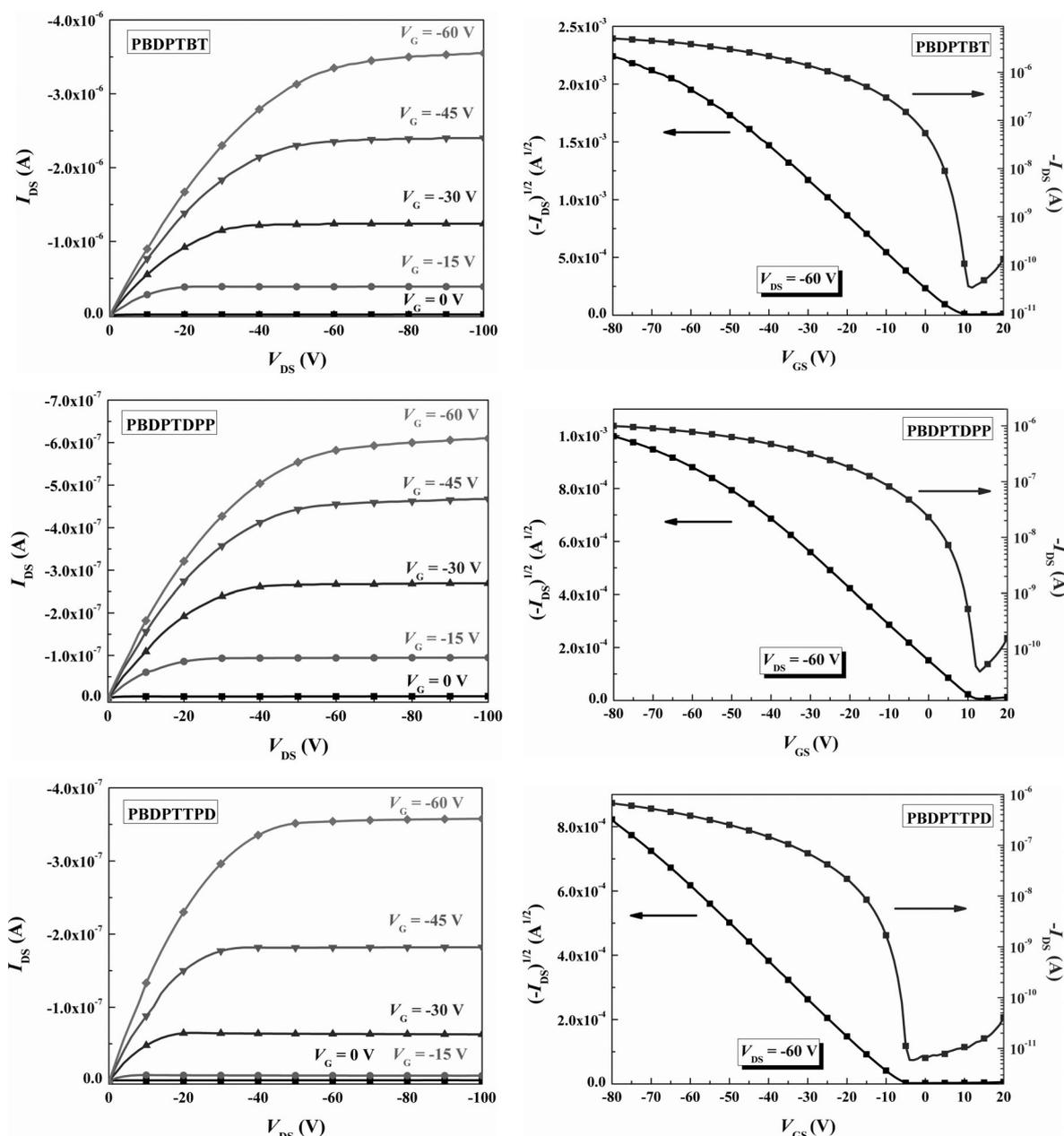
Figure 5. Typical output curves and transfer plots of the OFET devices based on **PBDPTBT** (top), **PBDPTDPP** (middle), and **PBDPTTPD** (bottom).
