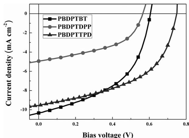
Figure 6. Current density–voltage characteristics of ITO/PEDOT:PSS/polymer:PC<sub>71</sub>BM/Ca/Al devices under illumination of AM 1.5 G at  $100 \text{ mW cm}^{-2}$ .
