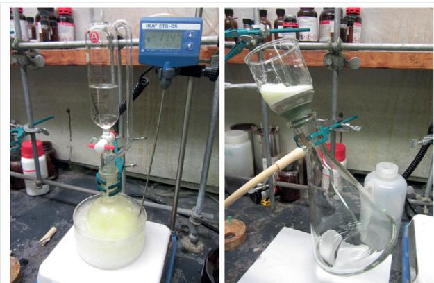
**Figure 2** (a) Reaction setup for hydrolysis of **3** and (b) filter flask setup that minimises the time required for filtration of **4** as fine particulates.
