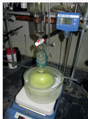
**Figure 1** Chlorination of *p*-iodotoluene by adding concd HCl to aqueous NaOCl and acetonitrile
