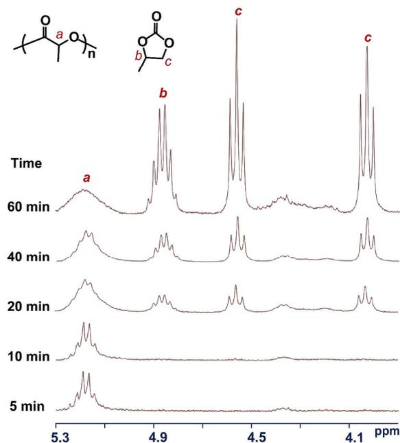
**Figure 3.**  $^1\text{H}$  NMR spectra recorded at regular intervals in  $\text{CDCl}_3$  during the reaction of Lac-OCA and PO in the presence of (salen)CoCl/[PPN]Cl. [PPNCl]/[I]=5; [OCA]/[I]=50.
