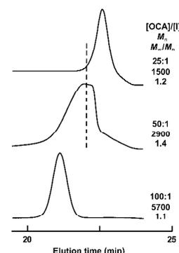
**Figure 1.** GPC curves of the polymers obtained by the ROP of Lac-OCA with (salen)CoCl/[PPN]Cl as the catalyst at different monomer-to-initiator ratios.
