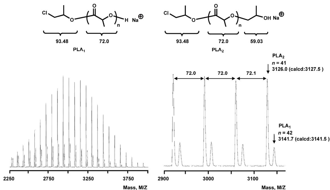
**Figure 2.** MALDI-TOF-MS spectra of polymers prepared by the ROP of Lac-OCA (Table 1, entry 8).
