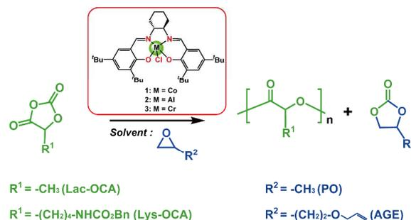
**Scheme 1.** Tandem synthesis of polyesters and cyclic carbonates catalyzed by metal salen complexes.
