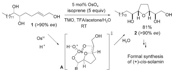
**Scheme 1.** Stereoselective oxidative cyclization of diols. TMO = Me<sub>3</sub>NO; TFA = trifluoroacetic acid.
