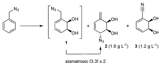
**Scheme 1.** Biotransformation of benzyl azide by *E. coli* JM109 (pDTG601) in a 5 L bioreactor by the previously described bi-phasic protocol.
