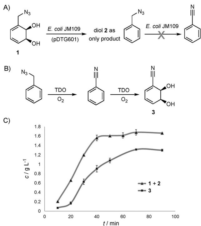
**Figure 1.** A) Diol **1** is not a substrate for TDO. *E. coli* JM109 does not oxidize benzyl azide to benzonitrile. B) Proposed sequence for the generation of diol **3**. C) HPLC product formation profiles for benzyl azide biotransformation in a 5 L bioreactor by using a biphasic protocol. Formations of diols **1** + **2** are expressed together to simplify data analysis.
