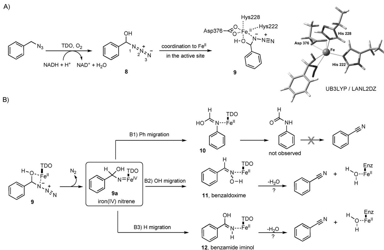
**Scheme 3.** A) Monooxygenation of benzyl azide by TDO gives hydroxyazide **8**, which could coordinate to Fe<sup>II</sup> in the active site of the enzyme. This bidentate coordination is supported by computational calculations at the UB3LYP/LANL2DZ level of theory. B) The proposed coordination could promote nitrogen loss to form an iron(IV)–nitrene complex, which could rearrange via three pathways (B1, B2 and B3).
