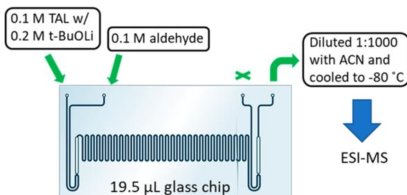
Figure 3. Microfluidic reactor schematic.
