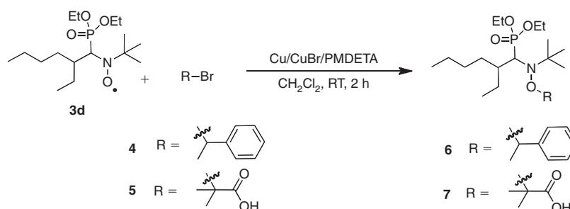
Scheme 3. Synthesis of  $\beta$ -phosphorylated nitroxide-based alkoxyamines.Table 3. Hyperfine splitting coupling constants of the different nitroxides in *tert*-butylbenzene ( $5 \times 10^{-4}$  M)
