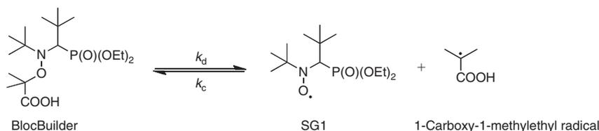
**Scheme 1.** Decomposition of the BlocBuilder MA alkoxyamine.
