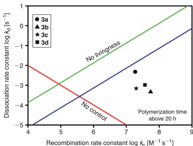
**Fig. 1.** Phase diagram for a the styrene polymerization at 120°C ( $k_p = 2050 \text{ M}^{-1} \text{ s}^{-1}$ ;  $k_t = 1.5 \times 10^8 \text{ M}^{-1} \text{ s}^{-1}$ ; [Alkoxyamine]<sub>0</sub> = 0.05 M; Limit criteria  $\Phi_{\text{lim}} = 0.3$ ,  $\delta_{\text{lim}} = 0.3$ , and  $t_{90} = 20 \text{ h}$ ).
