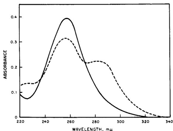
FIGURE 5: The ultraviolet absorption spectrum of monobenzoyleuracil. —, pH 6; -----, pH 11.5.
