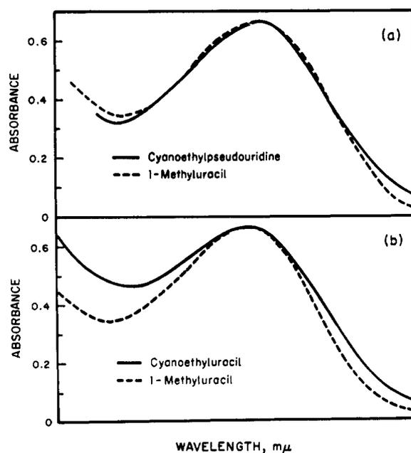
FIGURE 3: Ultraviolet absorption spectra of cyanoethylpseudouridine and cyanoethyluracil compared to 1-methyluracil. The 1-methyluracil spectrum (Shugar and Fox, 1952) was corrected so that its  $\lambda_{\max}$  and  $\epsilon_{\max}$  coincided with  $\lambda_{\max}$  and  $\epsilon_{\max}$  of cyanoethyluracil or cyanoethylpseudouridine.
