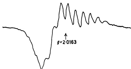
FIGURE 2. E.s.r. spectrum of sulphur containing 91.8% ^{33}\text{S} in 20% oleum. The solution contained ca. 0.2–0.3 mg S in 1 ml oleum.
