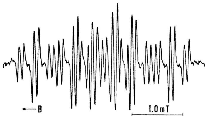
FIG. 2.—E.s.r. spectrum obtained *after* u.-v. photolysis of nitroterephthalic acid dissolved in tetrahydrofuran.
