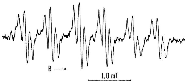
FIG. 4.—E.s.r. spectrum obtained *during* u.-v. photolysis at 233 K of 5-nitro-2-furaldehyde diacetate dissolved in tetrahydrofuran.
