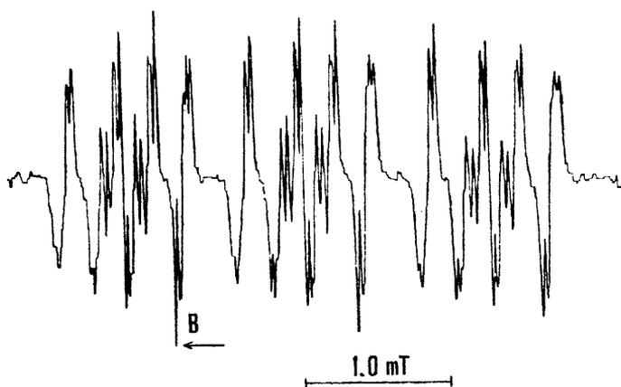
FIG. 5.—E.s.r. spectrum obtained during u.-v. photolysis at 278 K of 2-nitrothiazole dissolved in tetrahydrofuran.
