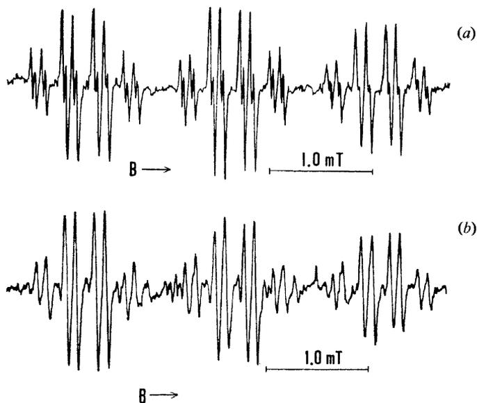
FIG. 1.—E.s.r. spectrum obtained *during* u.-v. photolysis of 3-nitrobenzoic acid dissolved in (a) tetrahydrofuran and (b) 2,5-dimethyltetrahydrofuran.
