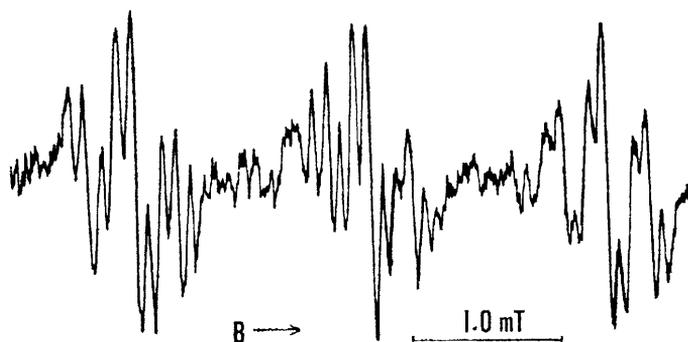
FIG. 3.—E.s.r. spectrum obtained *during* u.-v. photolysis at 278 K of 4-nitrophenol dissolved in 90 % v/v tetrahydrofuran + 10 % v/v di-tertiarybutyl peroxide.
