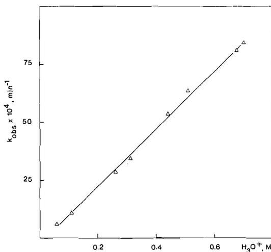
FIG. 1. Variation of the rate of appearance of the product **5** ( $R^1 = R^2 = \text{Me}$ ) with acidity (30 °C).
