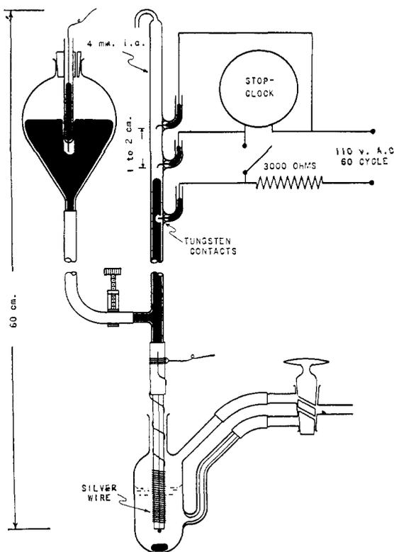
Figure 1. Polarographic Cell
