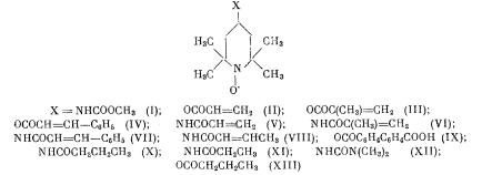
The new radicals were smoothly obtained by the selective reaction of 2,2,6,6-tetramethyl-4-hydroxyand of 2,2,6,6-tetramethyl-4-aminopiperidin-1-oxyls [14, 15] with the corresponding acid chloride in pyridine or triethylamine as medium. The compounds, self-contained radicals, were bright red crystalline substances, stable in air, readily distillable in vacuum without decomposition.
