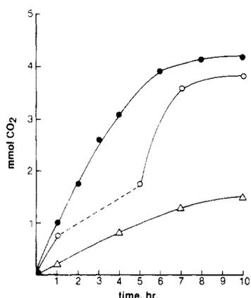
**Figure 1.** Oxidative decarboxylation of *N*-nitrosopyrrolidine without pyridine at 40 °C,  $\Delta$ . Pyridine-catalyzed decarboxylation at 40 °C under  $N_2$ ,  $\bullet$ . Catalyzed decarboxylation under  $O_2$ ,  $\circ$ --- $\circ$ ; continued under  $N_2$ ,  $\circ$ — $\circ$ .
