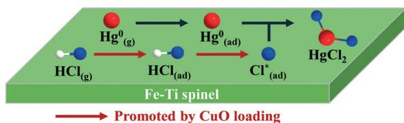
Fig. 9 Promotion mechanism of CuO loading for Hg<sup>0</sup> oxidation on Fe-Ti spinel.
