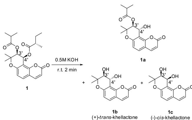
**Figure 1.** Partial and total alkaline hydrolysis of 1.
