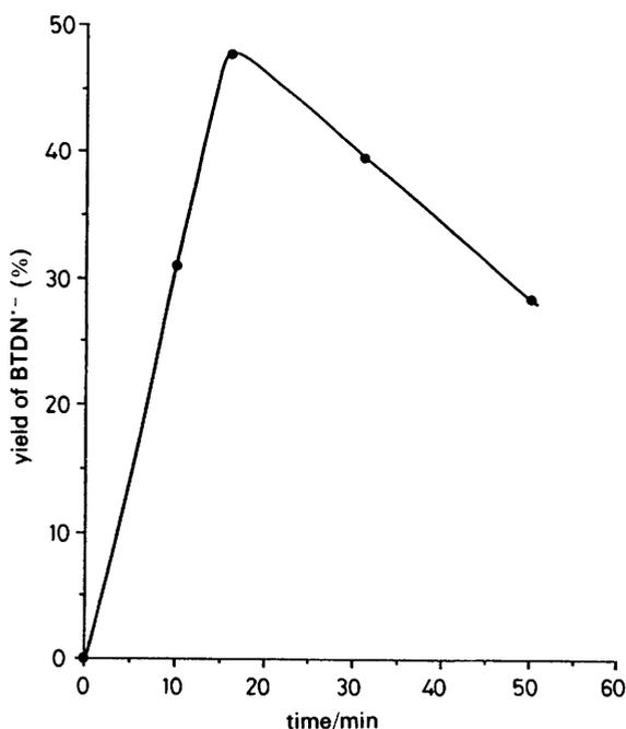
Fig. 1. Photogeneration of BTDN<sup>•-</sup> from BTDN ( $1.65 \times 10^{-4}$  mol dm<sup>-3</sup>), MES ( $0.05$  mol dm<sup>-3</sup>) and symmetrical DODAB ( $4 \times 10^{-3}$  mol dm<sup>-3</sup> vesicles).
