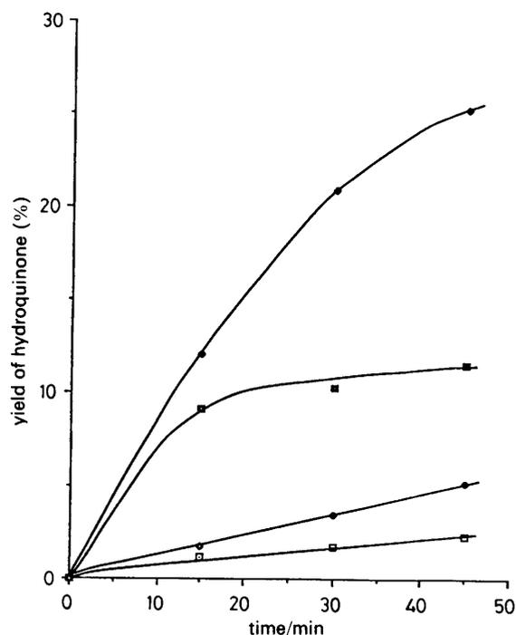
Fig. 3. Effect of [DODAB] in PC vesicles on the photochemical electron transfer from MES ( $0.05 \text{ mol dm}^{-3}$ ) in the inner water pools to 1,5-AQDS ( $1.65 \times 10^{-4} \text{ mol dm}^{-3}$ ) in the bulk water across vesicles, promoted by BTDN ( $1.65 \times 10^{-4} \text{ mol dm}^{-3}$ ). Total vesicle precursor concentration  $4 \times 10^{-3} \text{ mol dm}^{-3}$  (◆) PC : DODAB = 2 : 1; ◇ as ◆ but with light off; ■ PC : DODAB = 20:1; □ as ■ but with light off.
