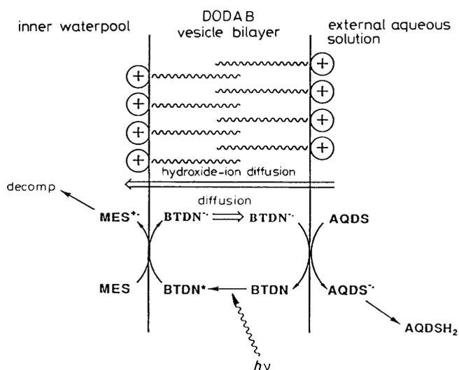
Scheme 1. Proposed mechanism for the transport of electrons from MES to 1,5-AQDS across bilayers of DODAB, mediated by BTDN.
