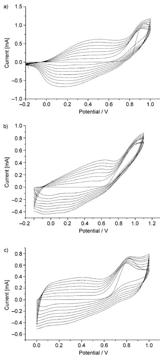
Figure 3. Electrochemical polymerization of pyrroles **7–9** by successive scanning over the first oxidation process in a  $10^{-3}$  M substrate and 0.1 M  $\text{LiClO}_4$  solution in acetonitrile, with Pt as working and auxiliary electrodes and  $\text{Ag}/\text{AgCl}$  as reference electrode.
