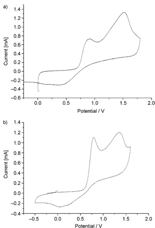
Figure 2. Cyclic voltammograms of pyrroles **7** and **9** in acetonitrile solution with  $10^{-3}$  M substrate and 0.1 M LiClO<sub>4</sub>, Pt as working and auxiliary electrodes, and Ag/AgCl as reference electrode.
