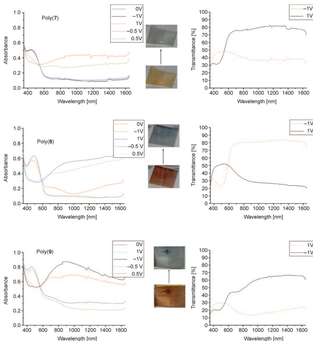
Figure 5. UV/Vis/IR spectroelectrochemistry (on the left) for poly(7)–poly(9) on indium tin oxide (ITO) plastic and the corresponding optical contrasts (on the right) for films obtained electrochemically applying the same number of scans (six cycles); Pt wire counter electrode, Ag/AgCl reference electrode, LiClO<sub>4</sub> supporting electrolyte (0.1 M).
