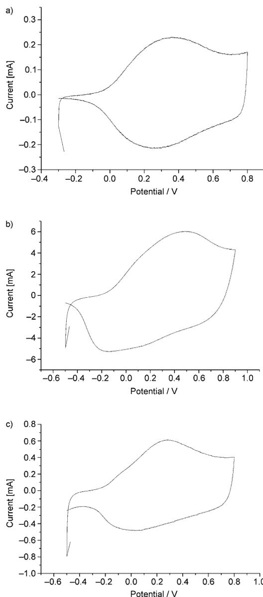
Figure 4. Cyclic voltammograms of a) poly(**7**), b) poly(**8**), and c) poly(**9**) in a monomer-free acetonitrile solution.
