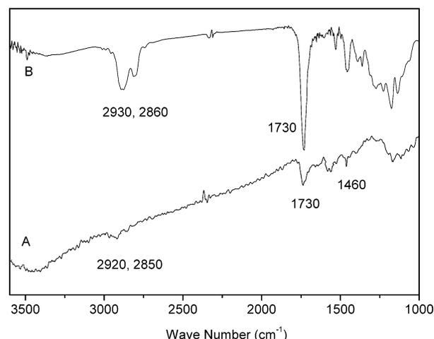
**Figure 1.** FT-IR spectra of multiwalled carbon nanotube (MWNT) surface grafted with COOCH<sub>2</sub>CH<sub>2</sub>OCOC(CH<sub>3</sub>)<sub>2</sub>Br group (MWNT-Br, A) and multiwalled carbon nanotube grafted with hyperbranched polymers 1 (HP-MWNT, B).
