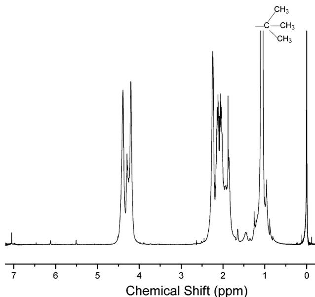
**Figure 6.** <sup>1</sup>H NMR spectrum of multiwalled carbon nanotube grafted with hyperbranched polymers containing *tert*-butyl acrylate units.
