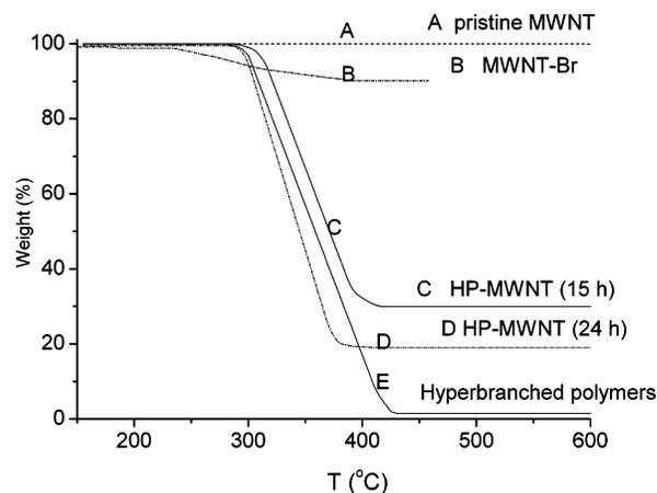
**Figure 2.** TGA curves of pristine multiwalled carbon nanotubes (MWNTs, A), MWNT-COOCH<sub>2</sub>CH<sub>2</sub>OCOC(CH<sub>3</sub>)<sub>2</sub>Br (MWNT-Br, B), MWNT grafted with hyperbranched polymers 1 (C, polymerization time was 15 h), MWNT grafted with hyperbranched polymers 2 (D polymerization time was 24 h), and hyperbranched polymers (E) under N<sub>2</sub>.
