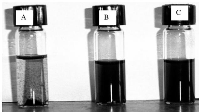
**Figure 4.** Solubility in organic solvent: MWNT-*g*-COOCH<sub>2</sub>-CH<sub>2</sub>OCOC(CH<sub>3</sub>)<sub>2</sub>Br in THF (A), MWNT grafted with hyperbranched polymers 1 in THF (B) and CHCl<sub>3</sub> (C).
