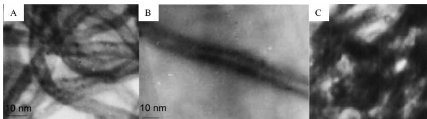
**Figure 5.** TEM images of MWNT-*g*-COOCH<sub>2</sub>CH<sub>2</sub>OCOC(CH<sub>3</sub>)<sub>2</sub>Br (A), MWNT grafted with hyperbranched polymers (B), and dispersion of MWNT-*g*-COOCH<sub>2</sub>CH<sub>2</sub>OCOC(CH<sub>3</sub>)<sub>2</sub>Br in hyperbranched polymer solution in THF (C).
