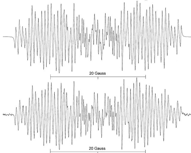
Figure 5. First derivative of the EPR spectrum recorded for a solution of  $[^{15}N]$ -**1a** in benzene (bottom) and spectrum simulated by using the hfc constants listed in Table 1 (top).
