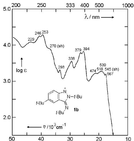
Figure 1. UV/Vis spectrum recorded for a solution of **1b** in heptane.
