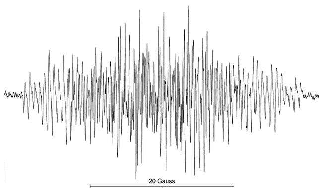
Figure 4. First derivative of the EPR spectrum recorded for a solution of  $[D_{18}]$ -**1a** in benzene.
