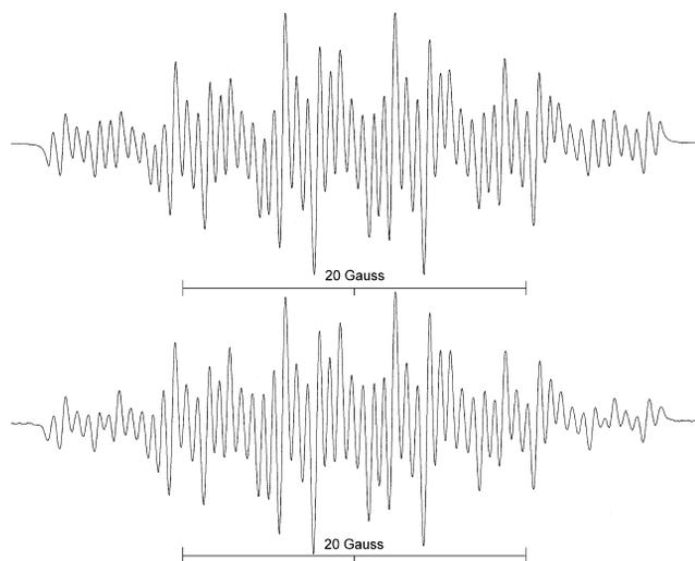
Figure 6. First derivative of the EPR spectrum recorded for a solution of **1b** in benzene ( $g = 2.0035$ , bottom) and spectrum simulated by using the hfc constants listed in Table 1 (top).
