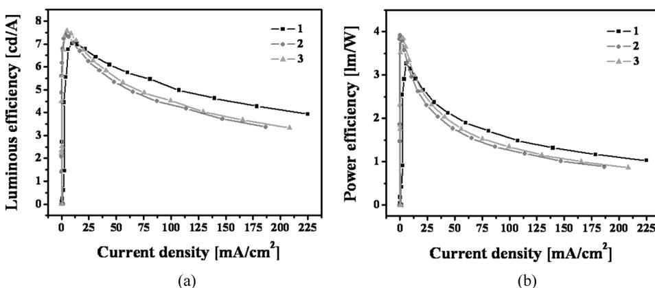
**Figure 5.** (a) Luminous efficiencies and (b) power efficiencies as a function of current density for the devices 1–3.
