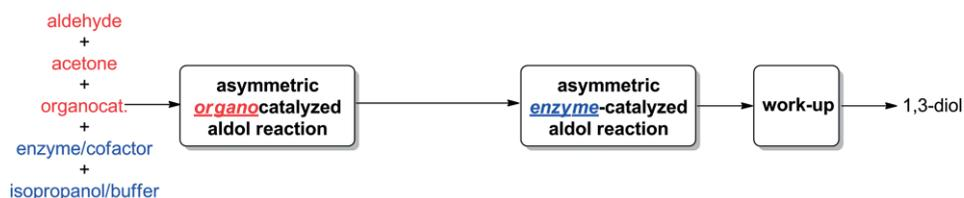
Scheme 2. Comparison of unit operations flow of the previously<sup>[5a]</sup> developed one-pot process based on two consecutive reaction steps with the tandem-type, one-pot process.
