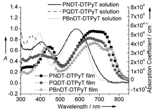
**Figure 1.** UV/Vis absorption spectra of PNDDT-DTPyT, PQDT-DTPyT, and PBnDT-DTPyT in chlorobenzene solution at 100 °C and in solid films.
