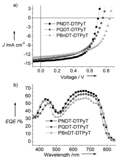
**Figure 2.** a) Current density–voltage ( $J$ – $V$ ) curves of polymer/PCBM-based solar cell devices under AM1.5G illumination ( $100 \text{ mW cm}^{-2}$ ). b) EQE curves of polymer/PCBM-based solar cell devices.
