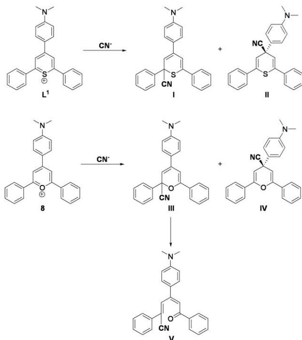
**Scheme 2** Proposed structures for the products of cyanide attack over thiopyrylium and pyrylium rings presented by receptors **L**<sup>1</sup> and **8**.
