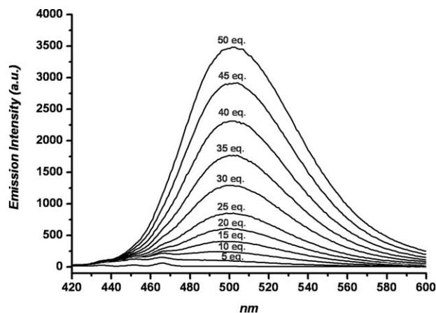
**Fig. 4** Emission enhancement observed upon addition of 50 equivalents of protons to acetonitrile solutions of  $L^1$  ( $1.0 \times 10^{-5}$  mol  $\text{dm}^{-3}$ ,  $\lambda_{\text{exc}} = 410$  nm).
