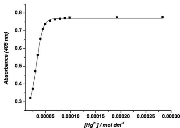
**Fig. 3** (Top) UV-visible spectra of  $L^5$  in acetonitrile ( $1.0 \times 10^{-5} \text{ mol dm}^{-3}$ ) and  $L^5$  in the presence of 10 equivalents of  $Hg^{2+}$  cation. (Bottom) changes in the visible band centred at 405 nm for receptor  $L^5$  upon addition of increasing quantities of  $Hg^{2+}$  cation.
