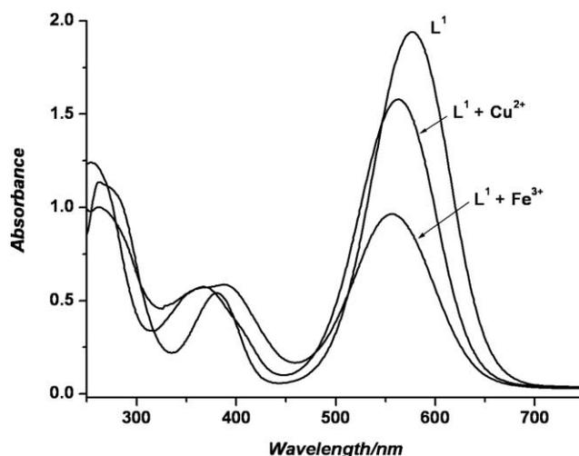
**Fig. 1** UV-visible spectra of  $L^1$  in acetonitrile ( $1.0 \times 10^{-5}$  mol dm $^{-3}$ ) and  $L^1$  in the presence of 10 equivalents of  $Fe^{3+}$  and  $Cu^{2+}$  cations.
