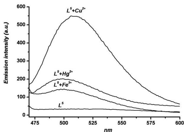
**Fig. 6** Fluorescence enhancements observed upon addition of 10 equivalents of the corresponding metal cations to acetonitrile solutions of receptor  $L^5$  ( $1.0 \times 10^{-5}$  mol  $\text{dm}^{-3}$ ,  $\lambda_{\text{exc}} = 410$  nm).
