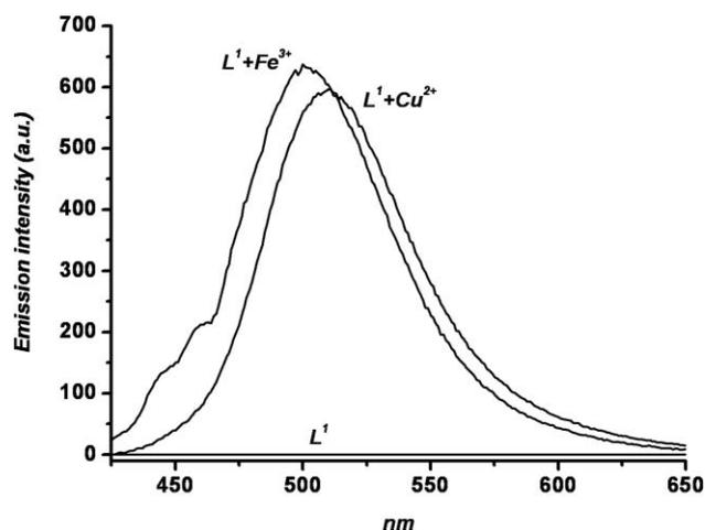
**Fig. 5** Fluorescence enhancements observed upon addition of 10 equivalents of the corresponding metal cations to acetonitrile solutions of receptor  $L^1$  ( $1.0 \times 10^{-5}$  mol  $\text{dm}^{-3}$ ,  $\lambda_{\text{exc}} = 410$  nm).
