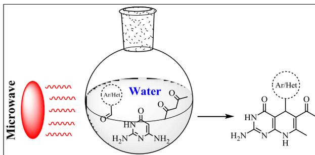
Three-component synthesis of 5-substituted 6-acetyl-2-amino-7-methyl-5,8-dihydropyrido[2,3-*d*]pyrimidines was brought to facile energy-efficient and environmental-friendly conditions using multicomponent reaction, microwave field as an activation method and hot water as a solvent. A series of the target compounds was synthesized using the developed procedure.
