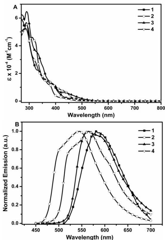
Figure 2. The absorption (A, 40  $\mu\text{M}$ ) and normalized emission spectra (B, 8  $\mu\text{M}$ ) of 1-4 in dichloromethane solution.  $\epsilon$  is the molar extinction coefficient.
