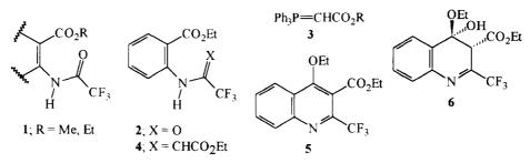
When ethyl 2-trifluoromethylamidobenzoate 2 was heated in the melt (180 - 200°) with carboethoxymethylenetriphenylphosphorane 3 (R = Et), the enamine 4 was not isolated but the quinoline derivative 5 was produced in 30 % yield.<sup>6</sup> Enamine 4 is evidently produced in the reaction but it undergoes
