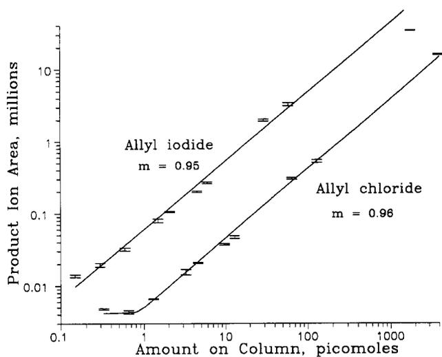
**Figure 10.** SRM calibration curves obtained by the reaction of the  $E^+$  ion of allyl chloride and allyl iodide with neutral pyridine in the collision cell. The error bars correspond to  $\pm 1$  standard deviation for triplicate injections.
