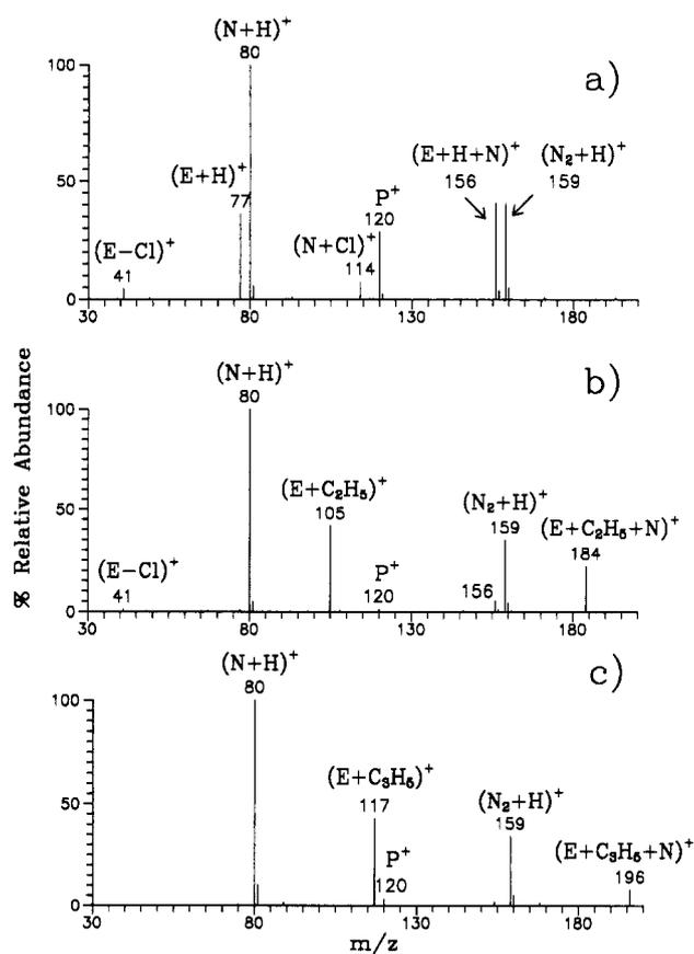
**Figure 9.** Mass spectra obtained by the reaction of neutral pyridine in the collision cell with the mass-selected (a)  $[E + H]^+$ , (b)  $[E + C_2H_5]^+$ , and (c)  $[E + C_3H_5]^+$  ions of allyl chloride.
