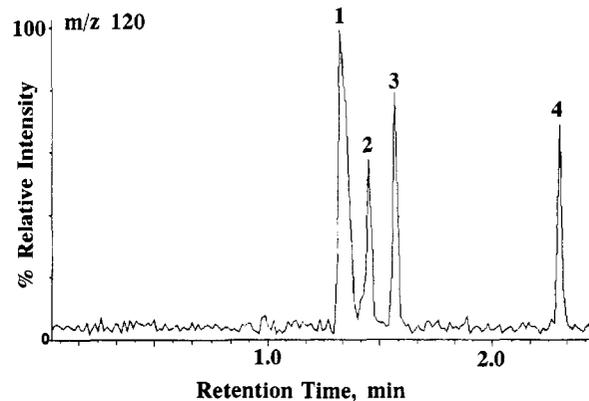
**Figure 6.** SRM mass chromatogram obtained by the reaction of the  $\text{N}^+$  ion of pyridine with 25 pg of allyl chloride (2) and allyl iodide (4). The peaks labeled (1) and (3) are due to the elution of pentane (solvent) and cyclopentane (impurity) into the collision cell.
