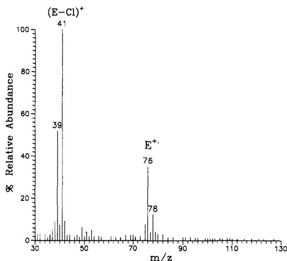
**Figure 7.** Q1MS mass spectrum of allyl chloride obtained with neutral pyridine in the collision cell.
