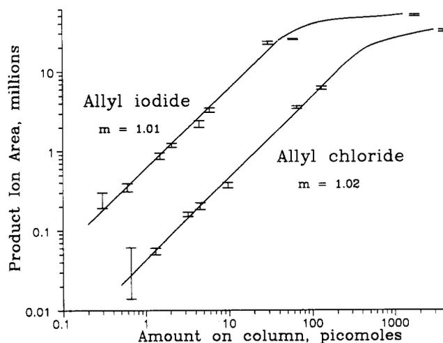
**Figure 12.** Full scan calibration curves obtained by the reaction of the  $E^+$  ion of allyl chloride and allyl iodide with neutral pyridine in the collision cell. The error bars correspond to  $\pm 1$  standard deviation for triplicate injections.
