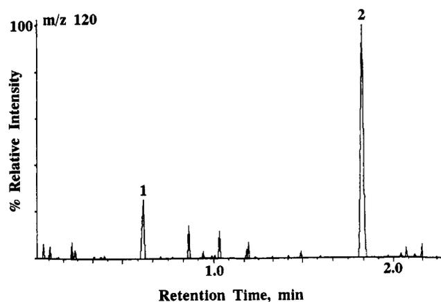
**Figure 13.** Full scan mass chromatogram ( $m/z$  120) obtained for the reaction of the  $E^+$  ions of 100 ng each of allyl chloride (1) and allyl iodide (2) solution with neutral pyridine in the collision cell.
