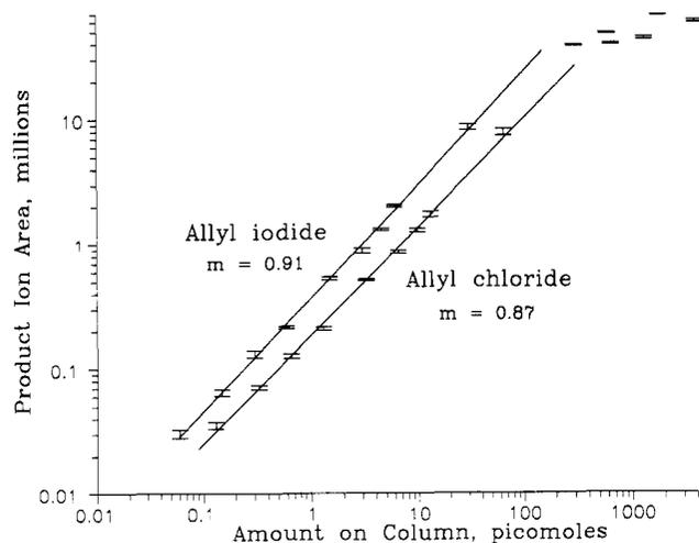
**Figure 5.** SRM calibration curves obtained for the reaction of the  $\text{N}^+$  ion of pyridine with allyl chloride and allyl iodide. The error bars correspond to  $\pm 1$  standard deviation for triplicate injections.
