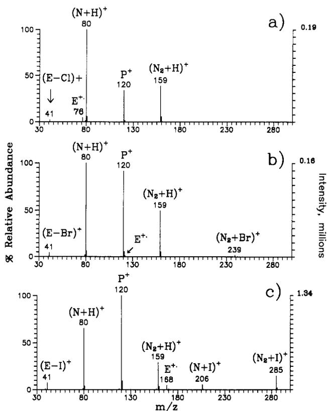
**Figure 8.** Mass spectra obtained by the reaction of neutral pyridine with the  $E^+$  ion of (a) allyl chloride, (b) allyl bromide, and (c) allyl iodide.
