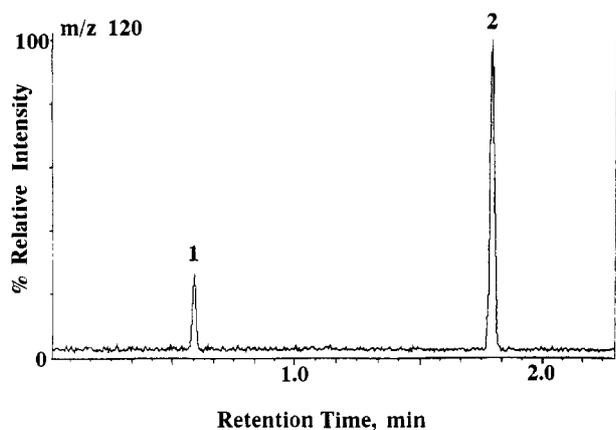
**Figure 11.** SRM mass chromatogram ( $m/z$  120) obtained for reaction of the  $E^+$  ions of 25 pg each of allyl chloride (1) and allyl iodide (2) solution with neutral pyridine in the collision cell. The signal/noise ratios were 6.0 and 23 for allyl chloride and allyl iodide, respectively.
