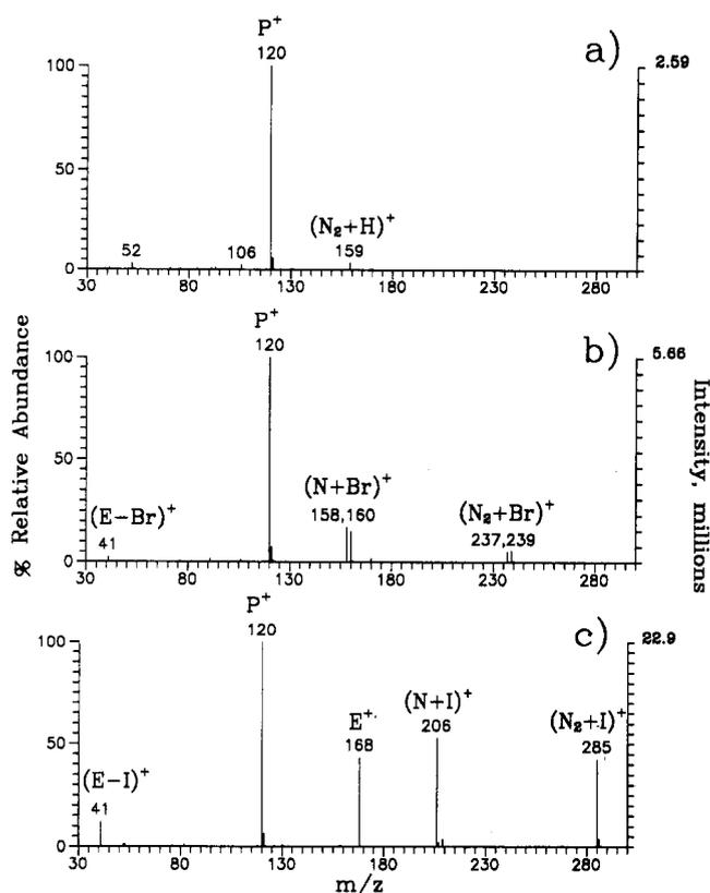
**Figure 3.** Background-subtracted mass spectra obtained from the reaction of the  $N^+$  ion of pyridine with (a) allyl chloride, (b) allyl bromide, and (c) allyl iodide.
