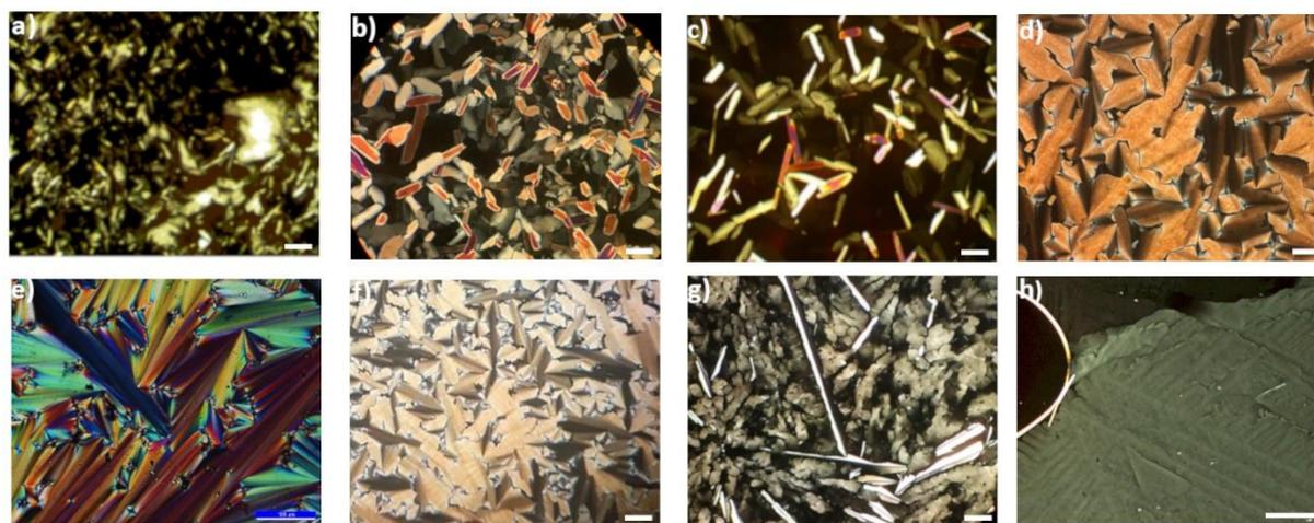
**Figure 1.** POM microphotographs obtained on cooling from the isotropic liquid. a) marble texture of **1.2bp14** at 53 °C; b) mosaic textures of **8.2bp7** at 92 °C; c) mosaic texture of **8.3bp8** at 165 °C; d) fan shaped texture of **8.2bp12** at 120 °C; e) fan shaped textures of **10.2bp16** at 190 °C; f) fan shaped textures of **10obp10** at 150 °C. g) dendritic textures of **12obp12** at 45 °C. h) dendritic textures of **14obp14** at 196 °C. The white&blue bars correspond to 100 μm.
