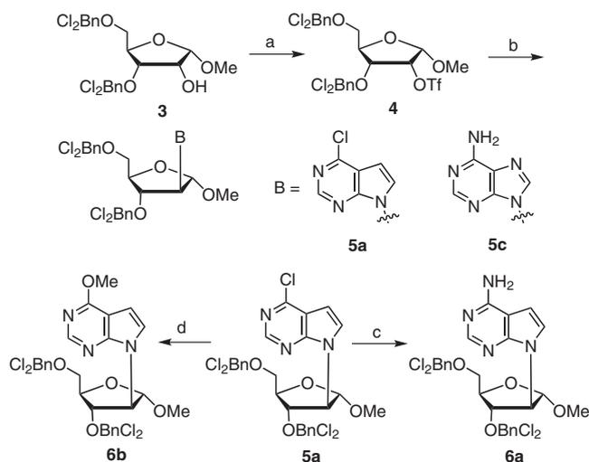
**Scheme 3** Reagents and conditions: (a) Tf<sub>2</sub>O, py, -40 °C to 0 °C (74%); (b) Cs<sub>2</sub>CO<sub>3</sub>, DMF, **5a** (87%), **5c** (79%); (c) NH<sub>3</sub>/MeOH, 120 °C, 12 h (77%); (d) NaOMe, r.t. 12 h (91%).
