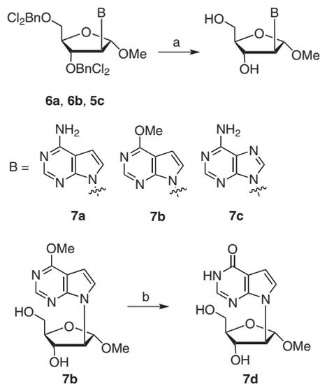
**Scheme 4** Reagents and conditions: (a) 20% Pd(OH)<sub>2</sub>, H<sub>2</sub>, Et<sub>3</sub>N, EtOAc, MeOH, **7a** (92%), **7b** (94%), **7c** (88%); (b) aq NaOH, reflux, 1.5 h (84%).
