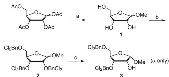
**Scheme 1** Reagents and conditions: (a) (i) NaOMe, MeOH, r.t.; (ii) Dowex-50w H<sup>+</sup> (87%), b/a 3:1; (b) 2,4-dichlorobenzyl chloride, NaH, DMF, 0 °C to r.t. (91%), b/a 3:1; (c) SnCl<sub>4</sub>, CH<sub>2</sub>Cl<sub>2</sub>, 0 °C, 28 h (85%).
