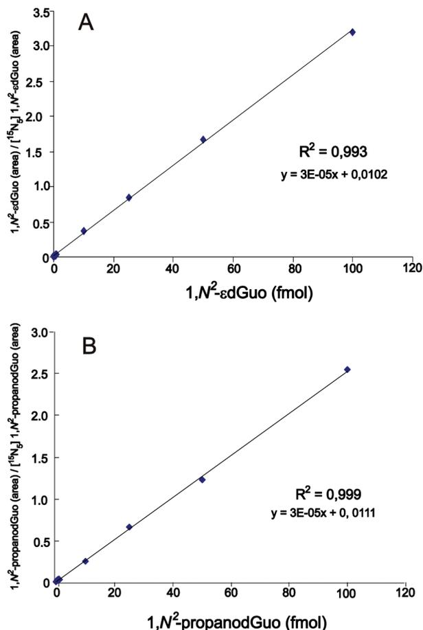
**Figure 3.** HPLC/ESI/MS-MS calibration curve for 1,N<sup>2</sup>-etheno-2'-deoxyguanosine (A) and 1,N<sup>2</sup>-propano-2'-deoxyguanosine (B), obtained by plotting the relative area ratios of unlabeled adducts to the isotopically  $^{15}\text{N}_5$ -labeled adduct vs increasing amounts of 1,N<sup>2</sup>-etheno-2'-deoxyguanosine and 1,N<sup>2</sup>-propano-2'-deoxyguanosine. Conditions were as described in the Experimental Procedures section.
