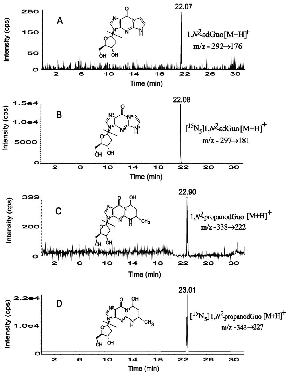
**Figure 1.** Detection of a 500 amol of DNA adducts standard by HPLC/ESI/MS-MS analysis in the MRM mode. (A)  $1,N^2$ - $\epsilon$ dGuo:  $m/z$  292  $\rightarrow$  176. (B)  $[^{15}\text{N}_5]1,N^2$ - $\epsilon$ dGuo:  $m/z$  297  $\rightarrow$  181. (C)  $1,N^2$ -propanodGuo:  $m/z$  338  $\rightarrow$  222. (D)  $[^{15}\text{N}_5]1,N^2$ -propanodGuo:  $m/z$  343  $\rightarrow$  227.
