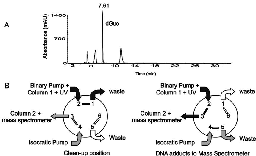
**Figure 2.** (A) Enzymatically hydrolyzed DNA;  $\lambda = 260$  nm. Conditions were as described in the Experimental Procedures section. (B) Positions of the automated switching valve during the HPLC/ESI/MS-MS analysis, cleaning and mass spectrometer positions.
