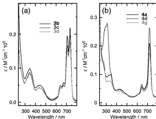
Figure 1. UV/Vis spectroscopy of a) clickable (**3a–3c**) and b) clicked Pcs (**4a**, **4d**, and **4g**).
