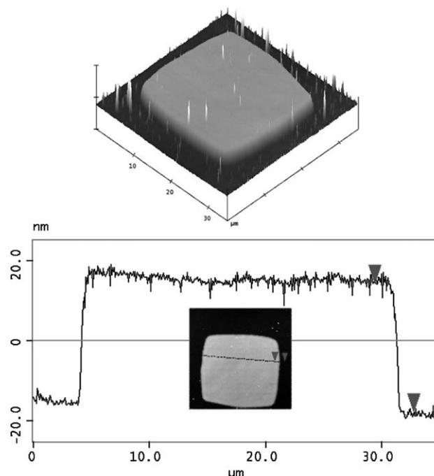
Figure 4. AFM images (full images in the Supporting Information) of patterned Pc **4d** showing 30  $\mu\text{m}$  square features in a thin film.
