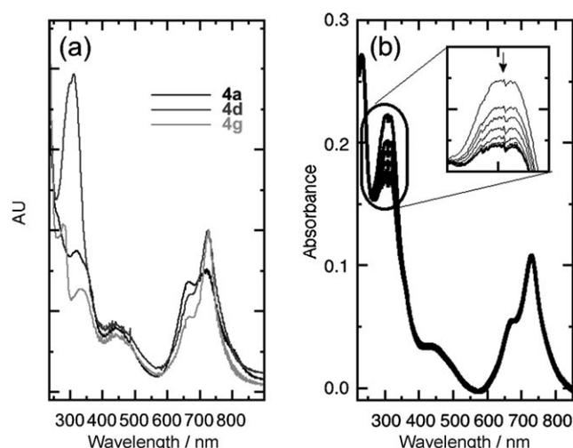
Figure 3. a) UV/Vis spectroscopy of thin films of clicked Pcs (**4a**, **4d**, and **4g**) spin-coated on quartz; b) UV absorption spectra of a spin-cast film of **4e** before, during (10 min intervals, 0→90 min), and after irradiation and wet development (bold trace).
